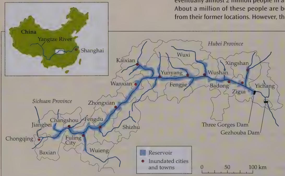
The Three Gorges Dam is flooding a 600 km stretch of the Yangtze River Valley in central China. Because the terrain comprises gorges, ravines, and mountain slopes, the resulting reservoir will be narrow and deep. (After Chau 1995.)
